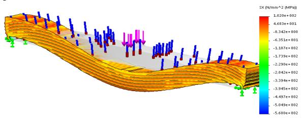
Fig. 8. Circuit of normal stresses in the prestressed glulam beam
