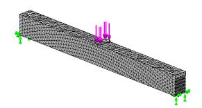
*Fig. 3.* Grid of finite elements of a straight-line beam patterned from pre-deformed lamellae Results and discussion
