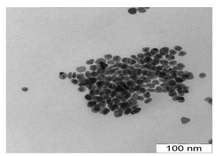
**Figure 1.** Silver nanoparticles (16 nm  $\pm$  5) according to TEM.
